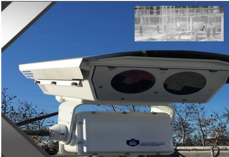
Thermal monitoring systems
